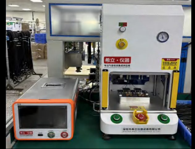
Air Leakage Waterproof
